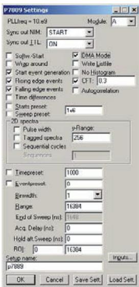
The Model P7889 is a 100 ps time bin, multiple-event time digitizer. It can be used in ultra-fast Multiscaler systems, in Time-of-Flight mass-spectrometry and time-resolved single ion- or photon counting.
