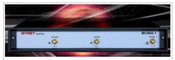
The MCS8A-1 is a 1+1 input multiple-event time digitizer. It detects the time of the incidence of the stop signals (rising, falling or both edges) relative to the start signal with 80 ps time resolution.
