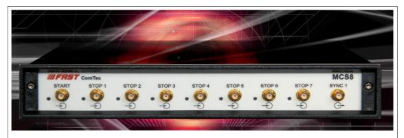
The MCS8 is a 7+1 input multiple-event time digitizer. It detects the time of the incidence of the stop signals (rising, falling or both edges) relative to the start signal with 80 ps time resolution.
