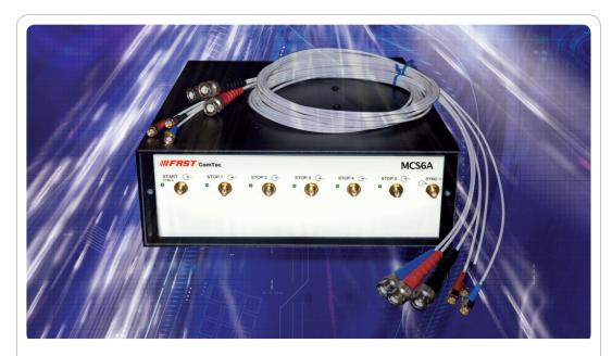
The MCS6A is a 5 input multiple-event time digitizer. It detects the time of the incidence of the stop signals (rising, falling or both edges) relative to the start signal with 100 ps time resolution.
