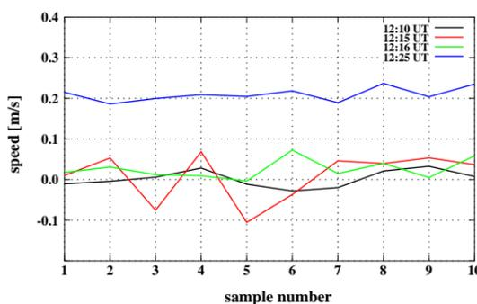
Figure 3: Apparent speed of the hard target vs. the laser system.
