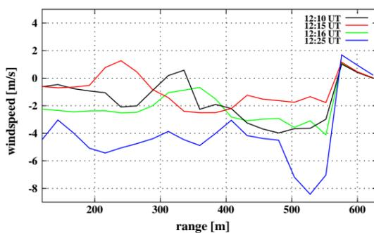
Figure 4: Horizontal wind speed profiles calculated from the measurements shown above.
