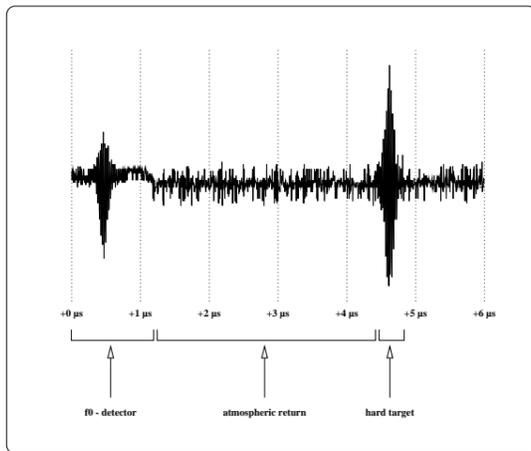
Figure 1: Example of a return signal from a hard target (single shot).
