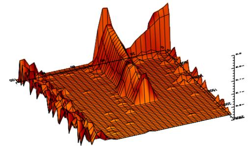
Figure 5: Profile of power spectra from a vertical measurement. The power spectra have been averaged over 15,000 shots ( $\approx 73$  seconds).
