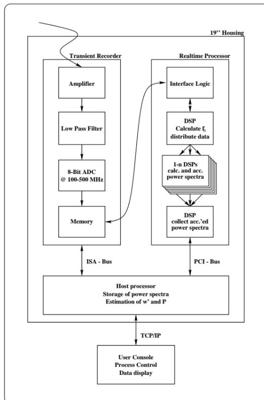
Figure 1: Layout of the data acquisition system hardware.
