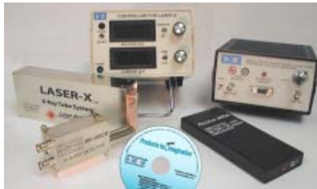
Figure 1: MCA8000A shown clockwise with Disk containing XRF-FP Quantitative Analysis Software and free MCA Software, Amptek XR-100CR X-Ray Detector, Amptek LASER-X X-Ray Generator, LASER-X Voltage and Current Controller and PX2CR Power Supply & Amplifier for the XR-100CR.
