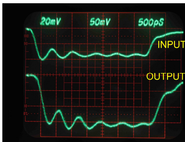
Fig. 1.2: Output pulseform (30 mV in, 150 mV out)
