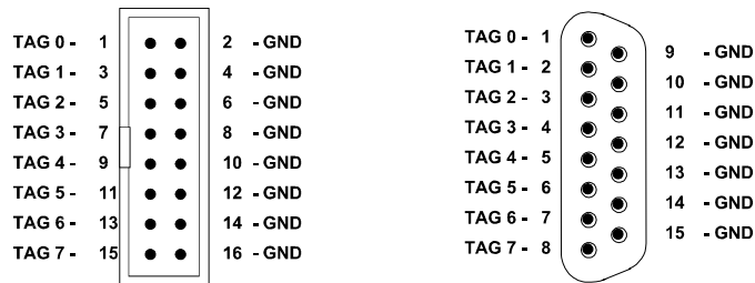
Figure 3.8: TAG input connector pinning
