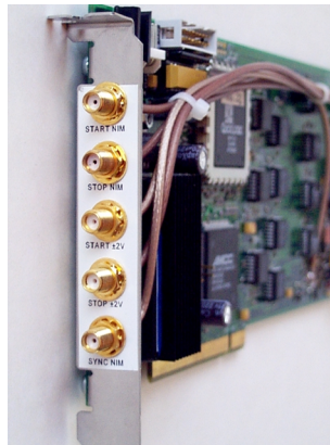
Figure 2.5: Bracket mounted signal connectors
