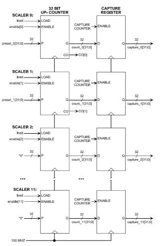
Figure 3.1: Simplified Block Diagram of Counters
