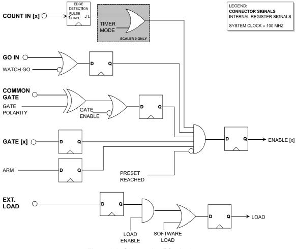
Figure 3.2: Schematic of Scaler Inputs
