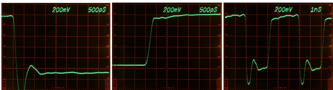
Fig. 8.10: SYNC_1 output signals 21 : fall time, rise time, 200 MHz clock
