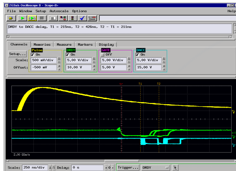
Fig. 8.17: ADC port handshake with 2 simultaneously firing ADC's
