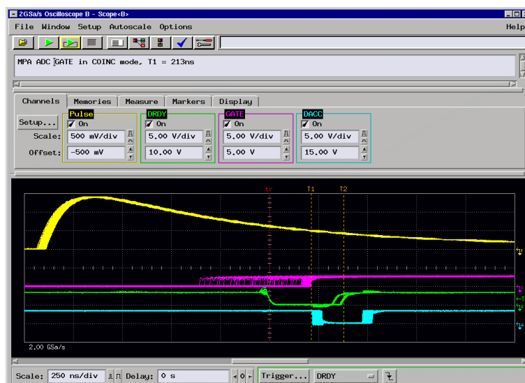
Fig. 8.19: ADC GATE setup time
