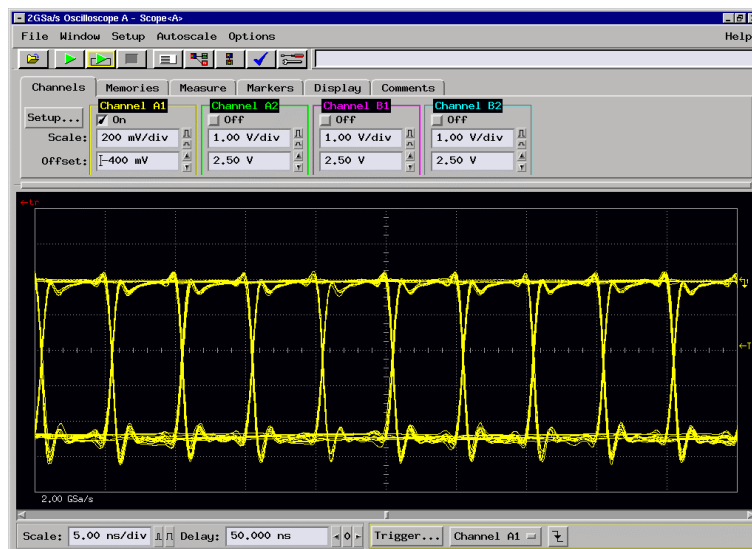
Fig. 8.15: Eye diagram using the PRBS output
