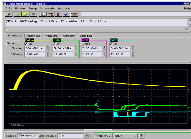
Fig. 8.5: ADC port handshake with 2 simultaneously firing ADC's
