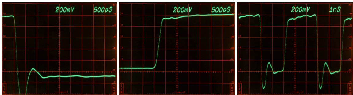
Fig. 8.9: SYNC_1 output signals 13 : fall time, rise time, 200 MHz clock
