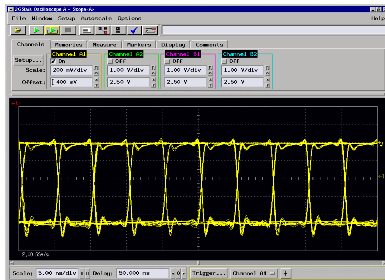
Fig. 8.14: Eye diagram using the PRBS output
