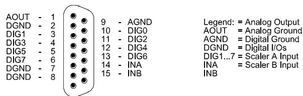
Figure 8.2: I/O port connector
