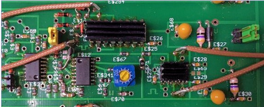
Fig.3: Potentiometer for setting the width of the TTL output pulses.
