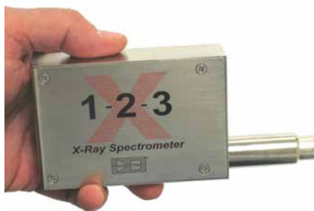
FIGURE 1. The CdTe detector in the X-123CdTe configuration
