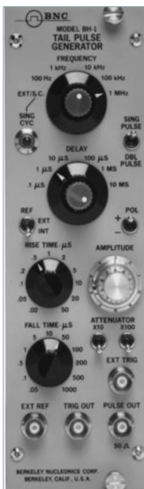
Fast Tail Pulser for simulating tail pulses as narrow as 5ns FWHM
