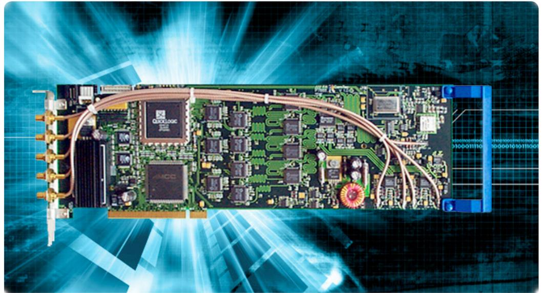
The Model P7888 Series are one of the fastest commercially available multiple-event time digitizers with up-to four inputs. They can be used as an ultra fast Multiscaler/TOF system in Time-of-Flight mass spectrometry and time-resolved single ion- or photon counting.
