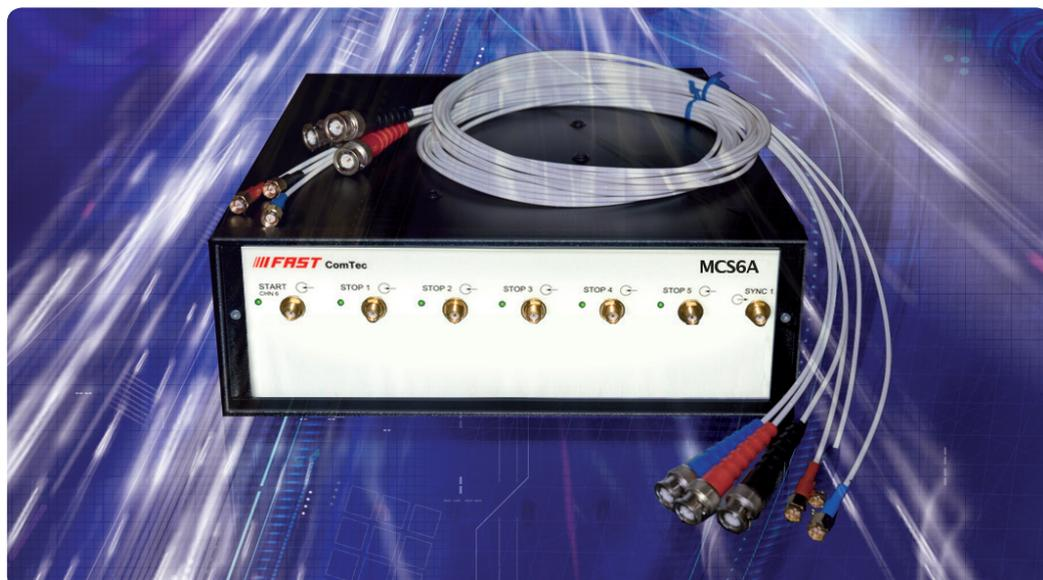
The MCS6A is a 5 input multiple-event time digitizer. It detects the time of the incidence of the stop signals (rising, falling or both edges) relative to the start signal with 100 ps time resolution.
