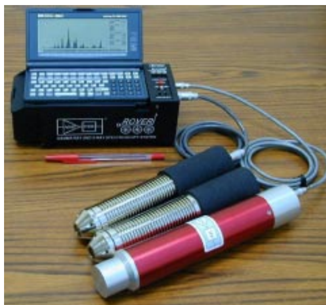
NaI detector shown here in a system with a SiPin-, CZT detector and an AMPTEK Rover System
